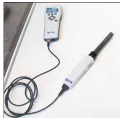
CO 2 air exchange testing equipment
