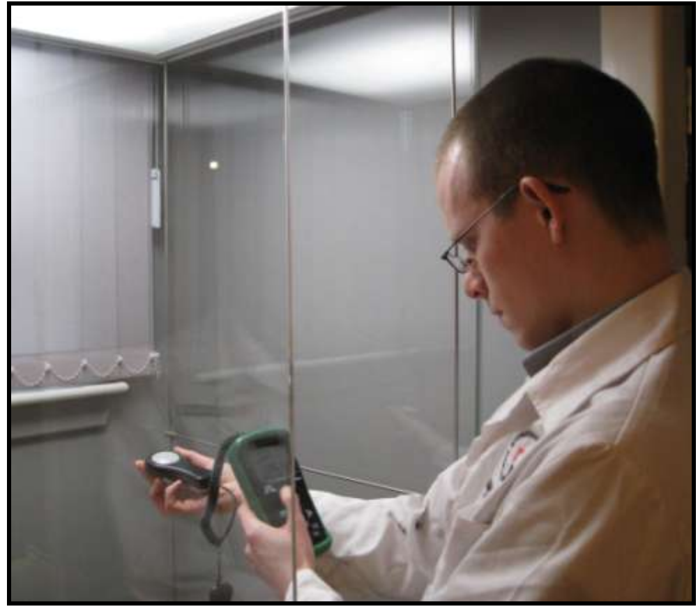
Measuring Lux Level of Lighting
